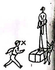
In case the hand chain pull force exceeds normal, don't pull by increasing force. Stop immediately and inspect the hoist
